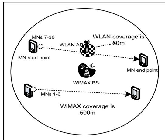
**Fig. 3.** Heterogeneous network scenario with 30 mobile terminals.
