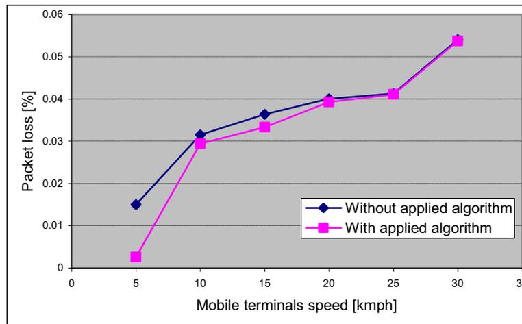
**Fig. 5.** Packet loss of the VoIP users with and without MS admission control algorithm in the WiMAX network.
