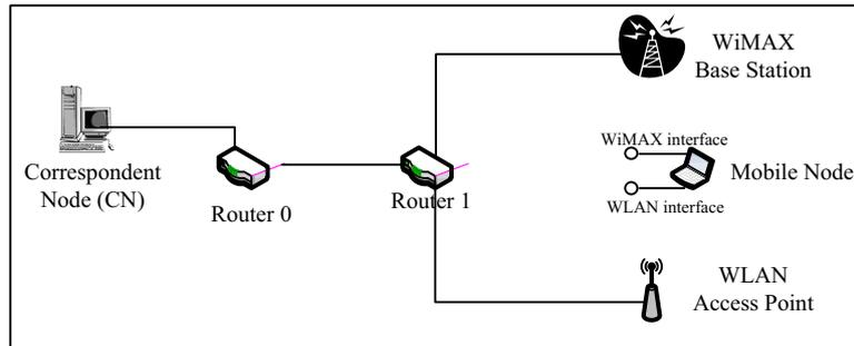
**Fig. 2.** Heterogeneous network topology.
