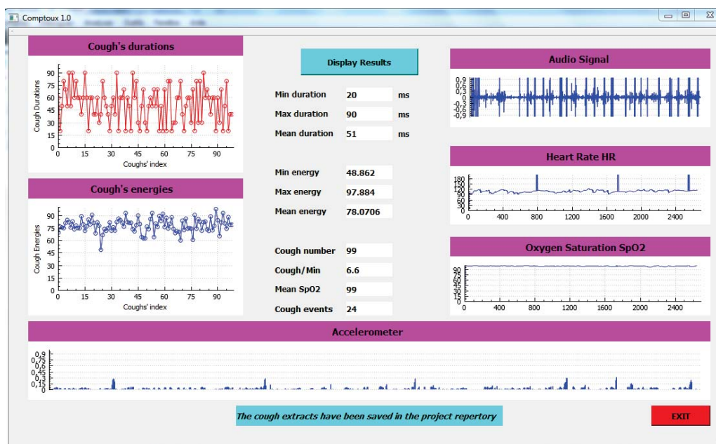
Fig. 4: Sensor-based Interface for Automatic Cough Detection.
