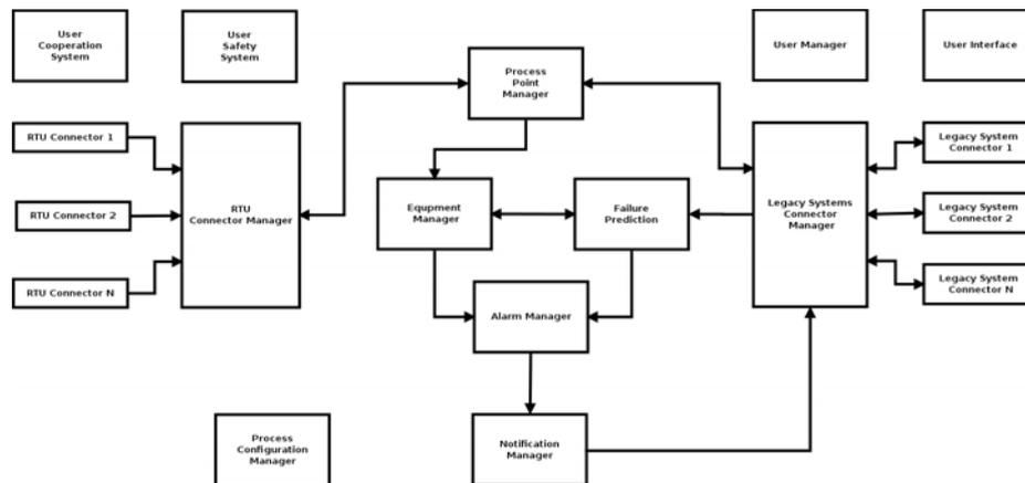
**Fig. 2.** Block diagram of the designed system
